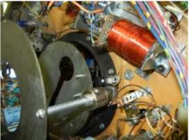
Loosen (DO NOT REMOVE) cannon mounting ring I had a screw covered by the below playfield ramp so I had to drop the ramp part way to access the screw.
