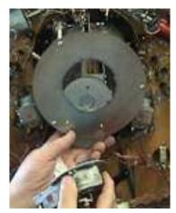
Remove 4 nyloc nuts securing the catapult to cannon assembly
