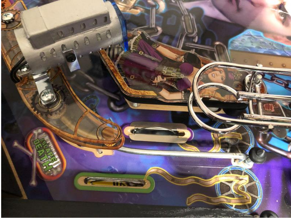
Right switch slot protector in place.
