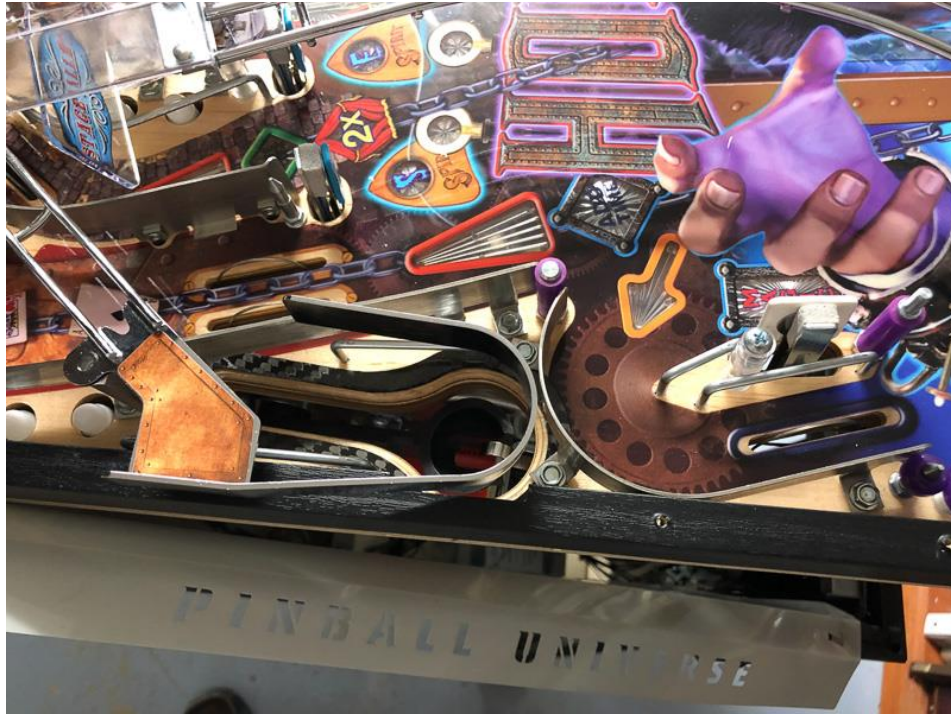
Milk can lane guide reinstalled. Also the rubbers to the right were all changed since they were easily accessible.
