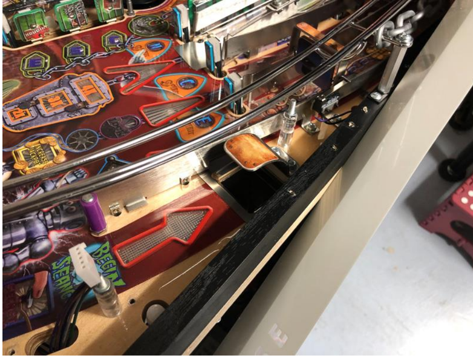
Left back post re-installed
