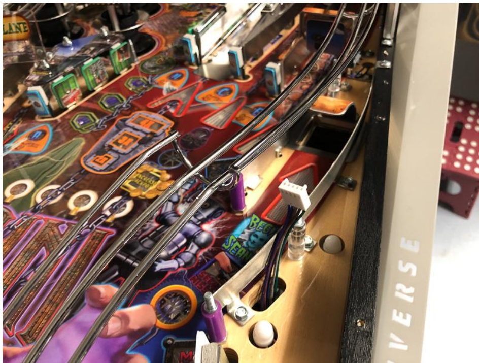
Right lane guide added back. Protector now snugly in place.
