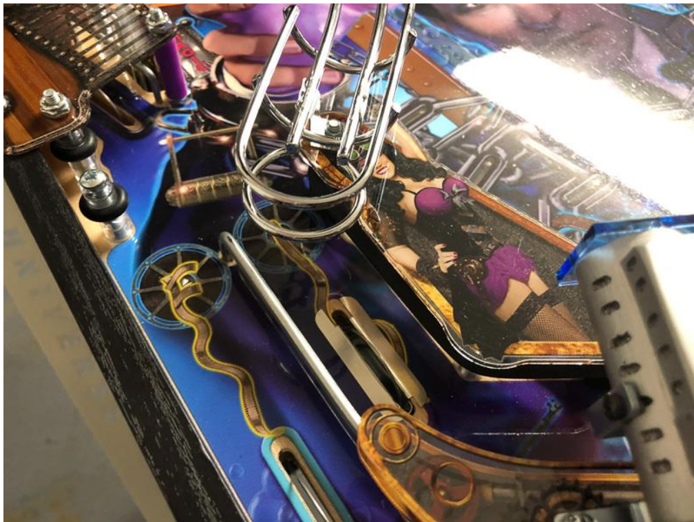
Left switch slot protector in place.
