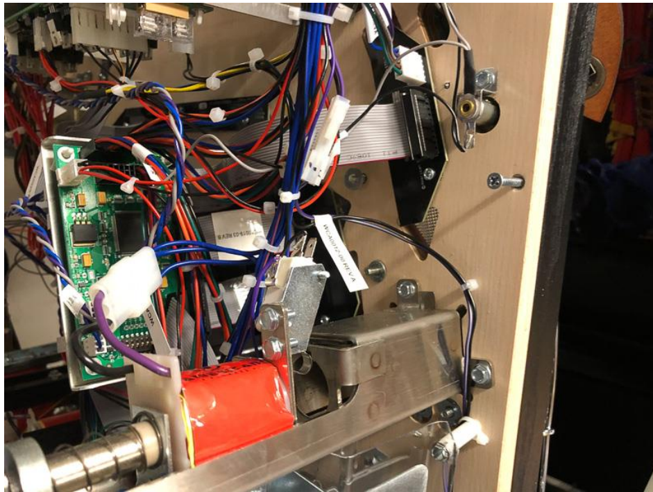
Tighten wood rail screws and re-install washers and nuts to left guide.
