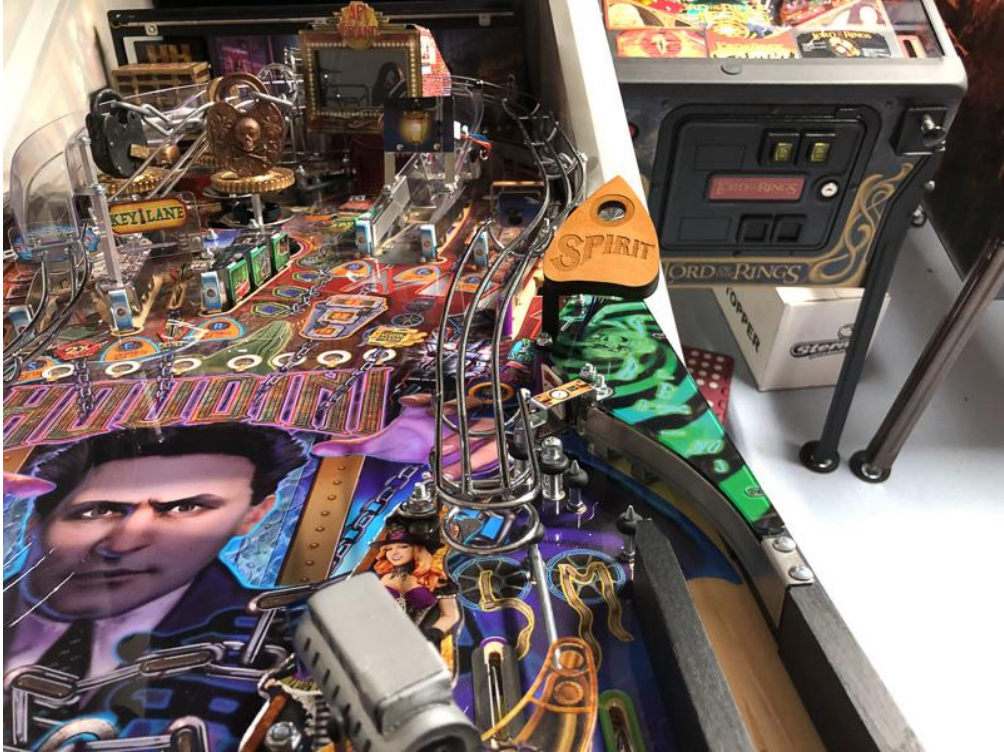
Unplug the Spirit light and remove the wood and the lower green/black plastic.
