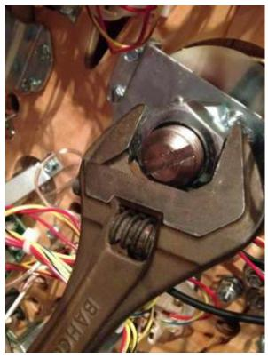
Now turn the magnet pole to raise it above playfield. One way lowers magnet, other way raises it. This can easily be felt with your fingers.
