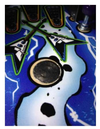
Locate magnet pole below playfield and loosen big lock nut
