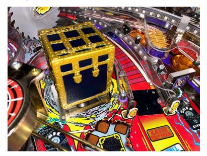
24. place the left mini-post back into the play field. Use a locking pliers to hold it in position.
