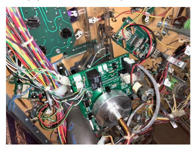
26. Lower the playfield. Time for testing! I tested the game in switch test mode and the eddy switch worked great. He protector has no ill effect. I tested the trunk movement and it moved smoothly and stopped correctly.
