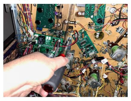
2. Remove the 2 remaining nuts at the bottom and the 1/4" hex bolt at the top left. (This is the bolt that goes into the T-nut to the right of the trunk.) [Before you remove the two nuts note the position of the trunk. The front of the trunk should be parallel to the front scoop.]
