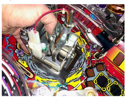
12. I lined up the protector and ensured post hole was centered and firmly pressed down on front where the 3M adhesive strip is. (make sure to wipe this area with the included alcohol swab just before installing)
