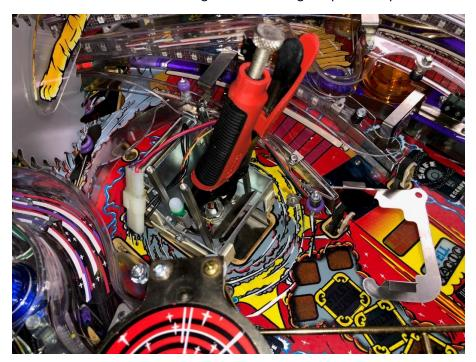
9. I aligned the right side of the protector first. I securely attached the lip on the right side.
