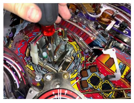
6. There are two large nuts holding the trunk to the underside assembly. The trunk assembly cannot be easily removed since there is a wire that would need a connector removed and I didn't want to do this much work.) As it turns out the assembly itself doesn't need to be removed. We just need to loosen the top section enough to slip the protector underneath
